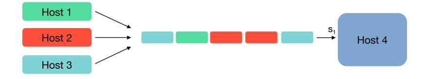
A server creates a socket to receive messages on a specific port number. Packets sent from different processes and/or systems all arrive on the same socket on the server
