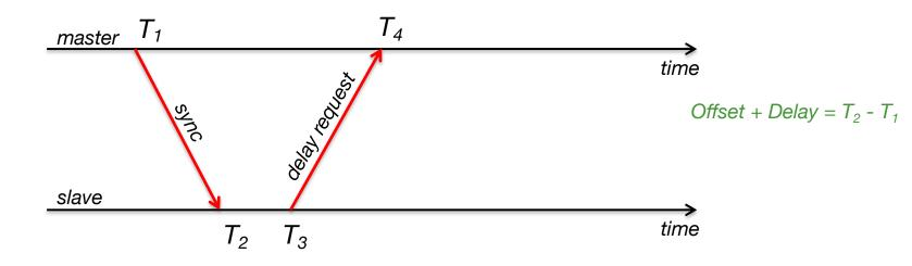
Slave needs to figure out the network delay. Send a *delay request*
