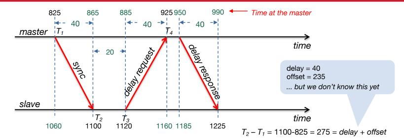
$master\_slave\_difference = T_2 - T_1 = delay + offset$   $slave\_master\_difference = T_4 - T_3 = delay - offset$  $master\_slave\_difference - slave\_master\_difference = 2(offset)$
