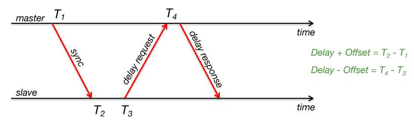
$$master\_slave\_difference = T_2 - T_1 = delay + offset$$
