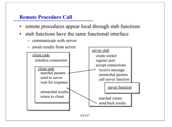
Remote procedure calls appear local because a local procedure exists that provides the same interface.
